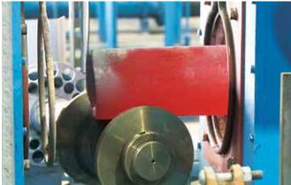
Our second ITTF operation is an all-induction line capable of processing a wider range of O.D. bars and tubes. The facility employs a unique V-shaped roll design that allows product to remain exceptionally straight. The piece-tracking system gathers key parameters at all points of processing.
